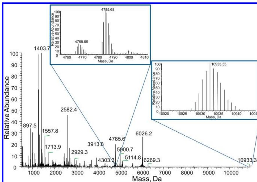
**Figure 6.** Fragmentation mass spectrum of pyruvate kinase monomer ejected from the intact tetramer complex. Pressure in the HCD cell was  $8 \times 10^{-10}$  mbar. The inset demonstrates fragment ion matches against the pyruvate kinase sequence at mass measurement accuracy better than 15 ppm.
