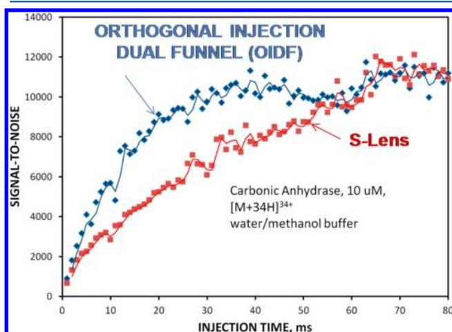
**Figure 2.** Signal-to-noise ratio as a function of the injection time into the C-trap for  $[M + 34H]^{34+}$  ions of bovine carbonic anhydrase at 10  $\mu\text{M}$  concentration. Signals were obtained with water/methanol/acetic acid buffer (49:49:2 v/v/v).
