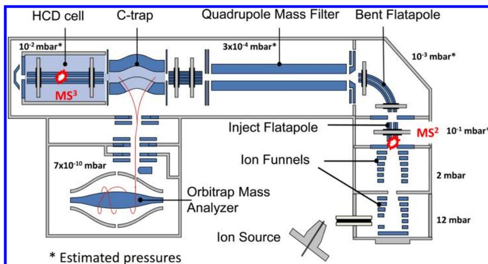
**Figure 1.** Schematic diagram of the modified Q Exactive mass spectrometer. The instrument encompasses a dual-funnel interface with orthogonal ion injection and quadrupole mass filter operating at a reduced rf-frequency of 285 kHz. Inject and bent flatapoles rf frequencies have been reduced to 2.6 MHz to improve higher  $m/z$  transmission.
