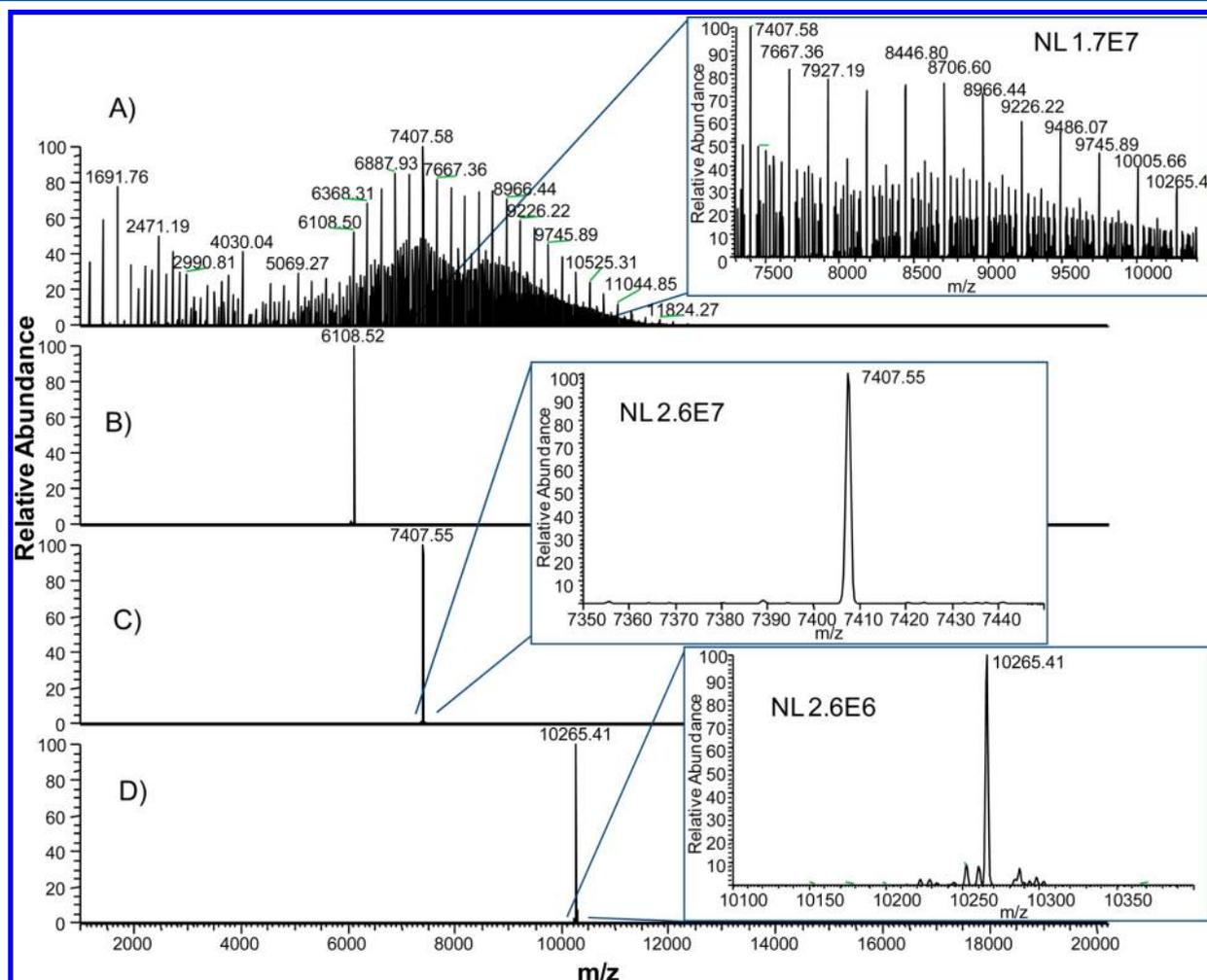
**Figure 3.** Full MS and quadrupole-selection mass spectra of aqueous solution of CsI at a concentration of 60 mg/mL obtained with the modified Q Exactive MS. Ion trapping was performed in the C-trap.
